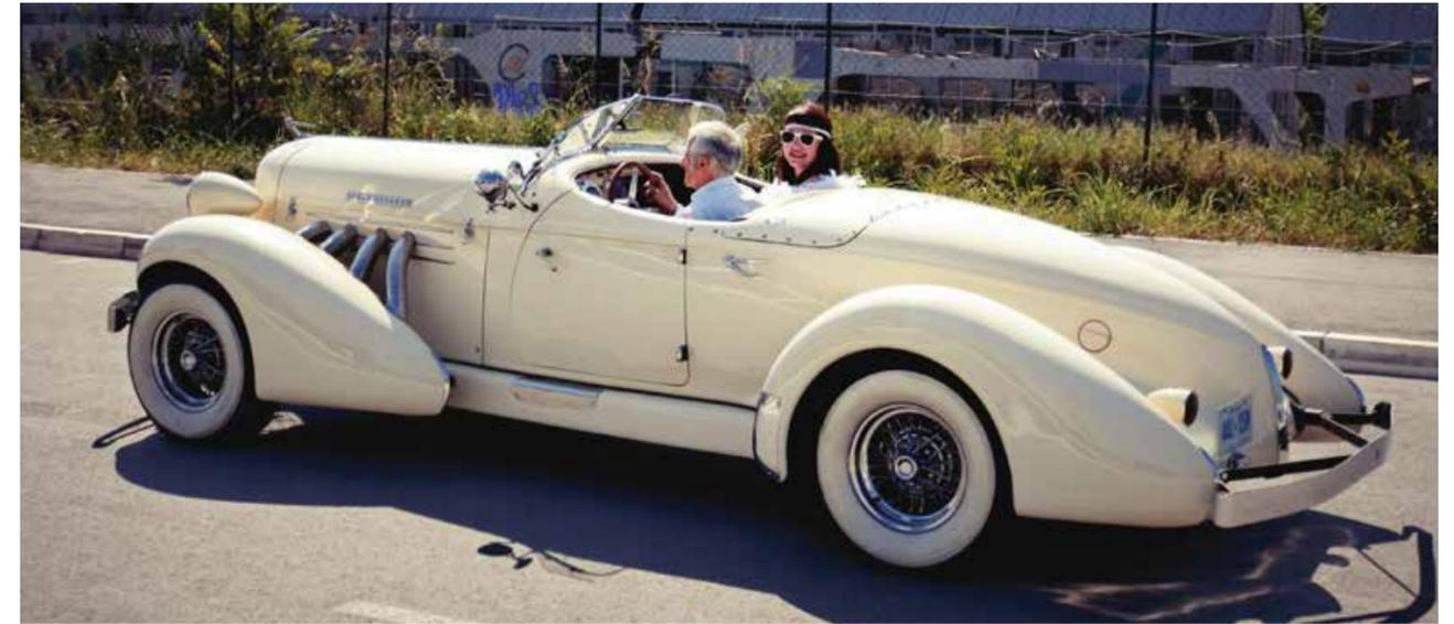
The Auburn 851 Speedster of 1935 was styled by designer Gordon Buehrig. The audacious 1935-1936 Auburn speedsters boasted curvaceous "boat-tail" bodywork on a potent supercharged eight-cylinder chassis, with a two-speed rear axle for relaxed highway cruising. A perfect storm of engineering and beauty, these cars combine elegance and modern drivability into an outstanding touring machine. The model has been referred to as the one genuine American
